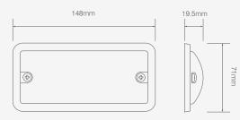
Overall Size: 148 x 71 x 19.5mm Cable Length: 200mm Current Draw (13.8V / 28V): 0.17A / 0.08A
